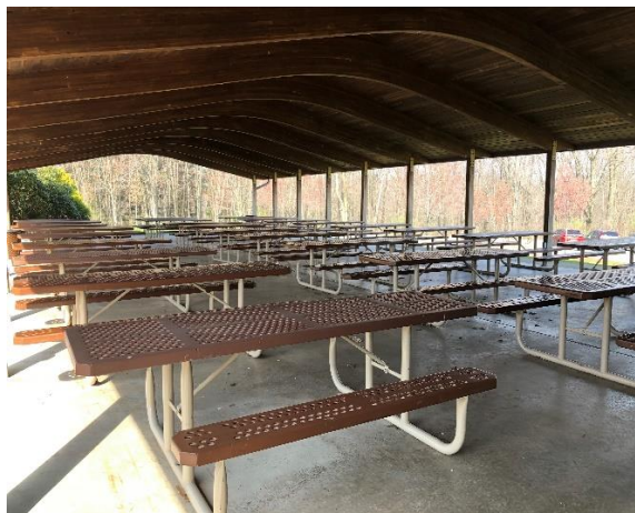
The table in the foreground has short benches to accommodate wheelchairs at the end.
